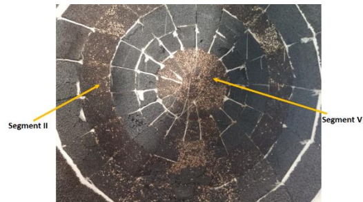
Figure 10. Details of the segments II and V of the cavity showing the colour change
