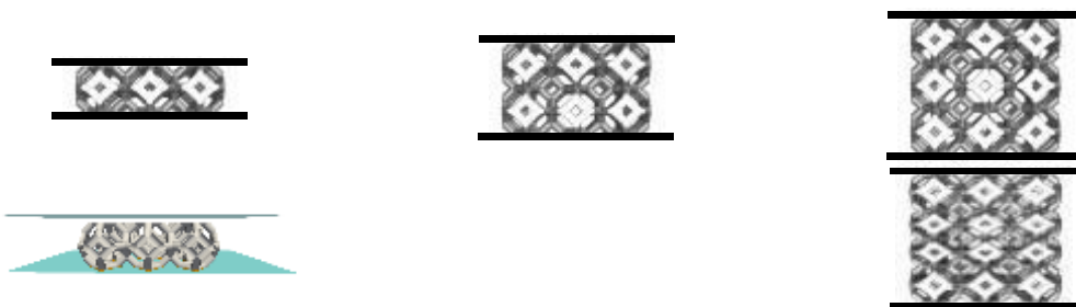
Figure 3. Frontal views of different Lattice core subdomains used for deriving correlations and study the radiation impact on the overall heat transfer
