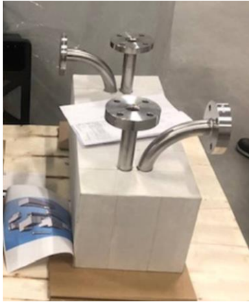
Figure 5. Prototype heat exchanger and insulation casing and parts for the covering of the ducts.
