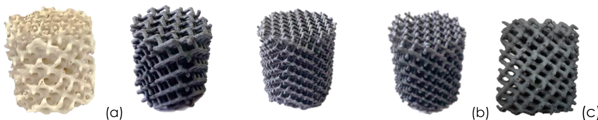
Figure 2. Novel lattice redox structures based on (a) \text{CeZrO}_2 , (b) \text{NiFe}_2\text{O}_4 for water splitting and (c) \text{Co}_3\text{O}_4 for \text{N}_2 purification via O-trapping respectively
