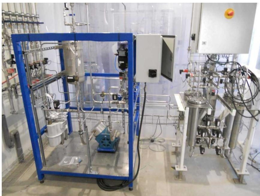
**Figure 5.** PSA test rig: 4-vessel PSA (right part of picture), vacuum pump and storage vessel (left part of image)
