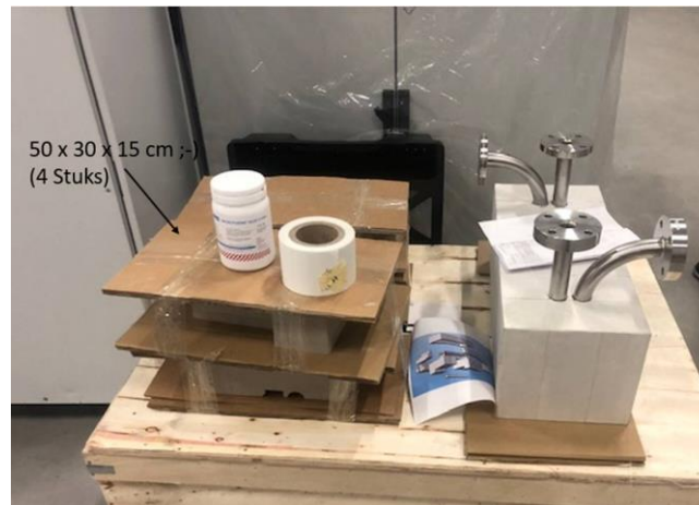
Figure 4. Prototype heat exchanger and insulation casing and parts for the covering of the ducts.
