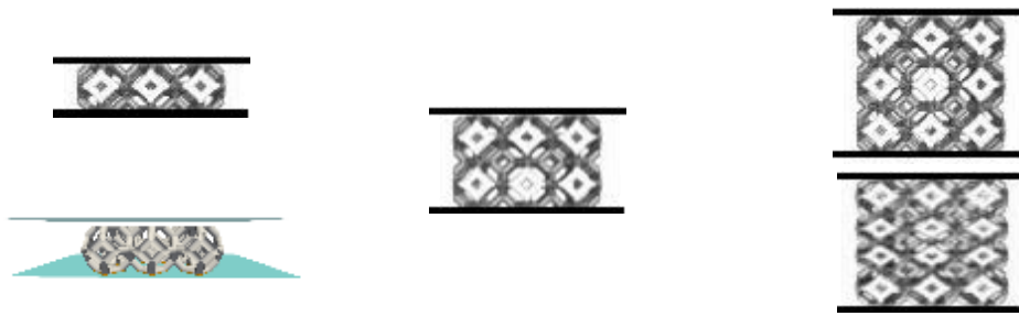
Figure 2. Frontal views of different Lattice core subdomains (1-3 layers, with and without gap, uniform and non-uniform cell size) used for deriving correlations and study radiation and its impact on the overall heat transfer
